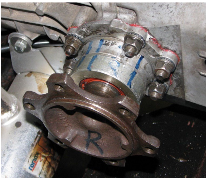
Photo 5: Another view of the gearbox output hub, showing the hub and its mounting flange which is held on the gearbox by six studs, nuts and star washers. A thin paper gasket (with gasket sealant on both sides) fits between the hub mounting flange and the gearbox face. The excess gasket sealant is shown in orange at the upper part of the photo.
