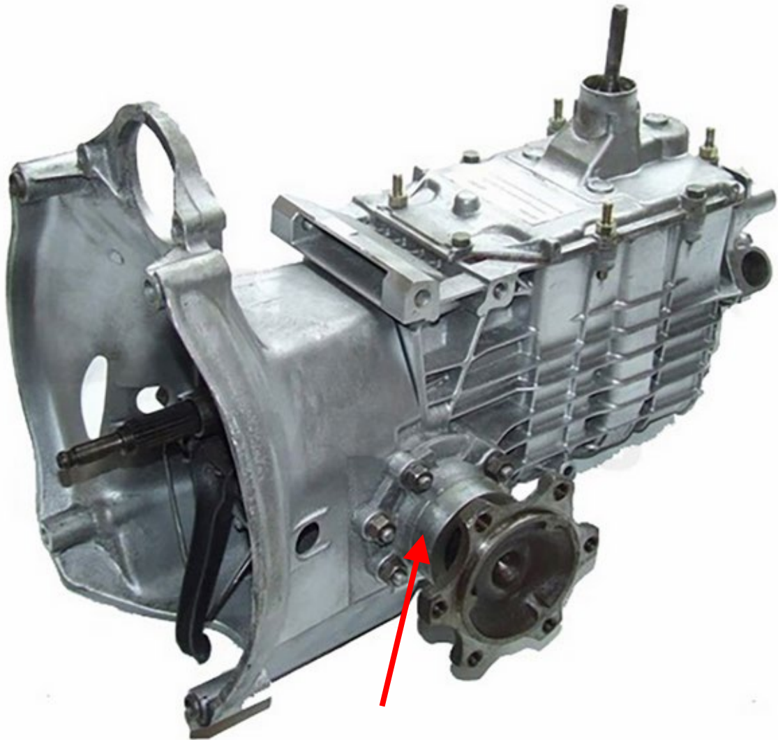
2CV Gearbox showing the left-side output hub (arrowed)
